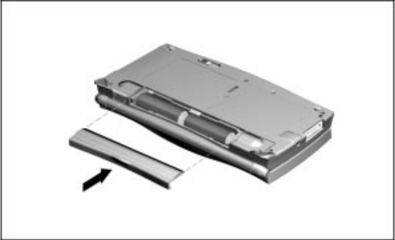
Replacing the Main Battery Cover
