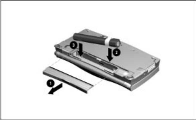
Installing the NiMH Battery Pack
