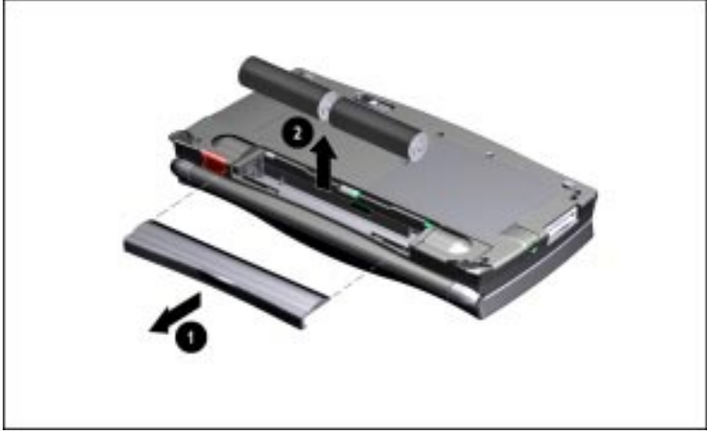
Removing the Old Main Batteries
