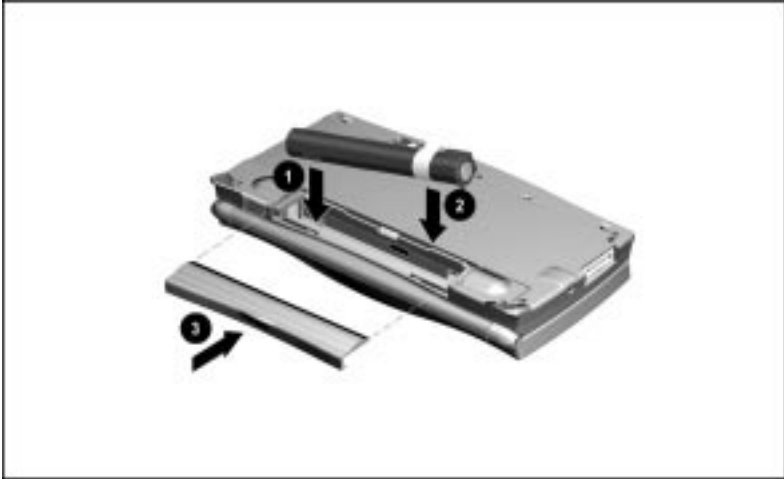
Installing the NiMH Battery Pack
