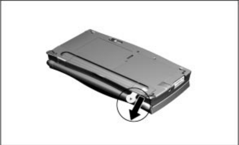
Removing the Backup Tape
